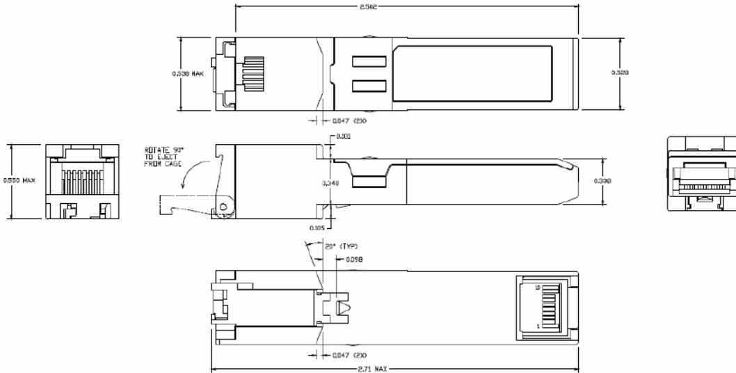
Figure 2. SFP24-(G)T mechanical dimensions
